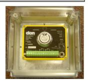
AARO-KJ fitted in an IP65 enclosure and certified to ATEX Cat 3 Zone 22 environment. The AC supply to the control unit and the field sensor input are pre wired to rail mounted fuses and feed through terminals.The enclosure is also fitted with an "Isolate elsewhere before removing the cover" warning label.
