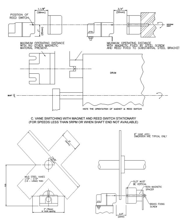
A. MAGNET MOUNTED ON SHAFT  $\mathbb{Q}_{-}$  (REED SWITCH GIVES 2 PULSES/REV)
