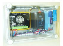
AARO rotation sensor control unit is housed in a GRP box, comprising: IP65 box of approximate dimensions 190h x
