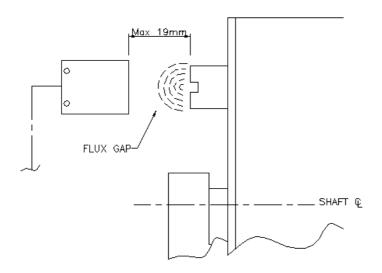
2 MAGNETS FITTED TO ROTATING DRUM DIAMETRICALLY OPPOSED PRODUCE 2 PULSES / REV.
