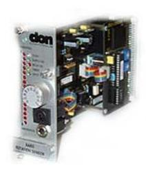
The rack mounted AARO has the same specification as the AA4406 housed in a 19" eurocard rack. It has an optional Modbus communication module for use with distributed control systems and SCADA packages. It also has the capability to incorporate other fieldbus communication protocols such as Profibus and DeviceNet.
