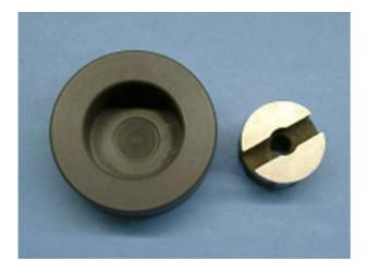
The MG1050 is a powerful permanent magnet 38mm in diameter with a 8mm fixing hole. The magnet can be mounted on the end of a rotating shaft or drum and is used in conjunction with a reed switch sensor (SR0421) or a Solid State Sensor (SR0531).
