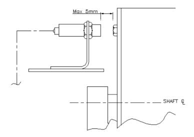
2 BOLT HEADS PROJECTING FROM ROTATING DRUM DIAMETRICALLY OPPOSED PRODUCE 2 PULES / REV
