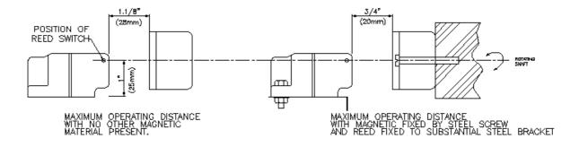
B. MAGNET MOUNTED ON FACE OF DRUM (REED SWITCH GIVES 1 PULSE/REV)
