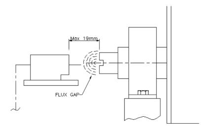
MAGNET FITTED TO ROTATING SHAFT ON CENTRE LINE AND PRODUCES 2 PULSES / REV.
