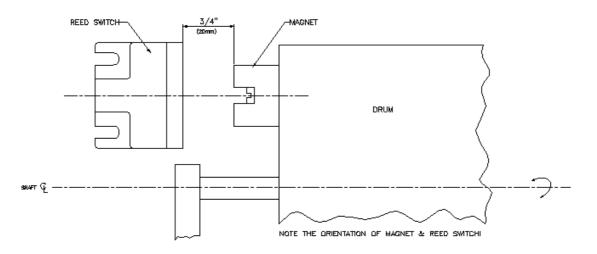
C. VANE SWITCHING WITH MAGNET AND REED SWITCH STATIONARY (FOR SPEEDS LESS THAN 5RPM OR WHEN SHAFT END NOT AVAILABLE)
